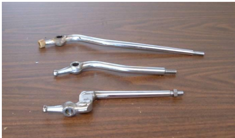
TOP – Stock Datsun 210 Gearshift Lever MIDDLE – Modified Lever by Cut-down and Tap Threads BOTTOM – Modified Lever by Cut and Weld
